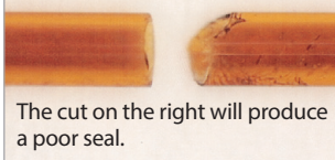
Figure 1: Make a clean, square cut for optimum connector performance.
